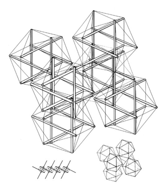
Fig. 784.41 Indefinitely Extensive Array of Tensegrity Icosahedra.
