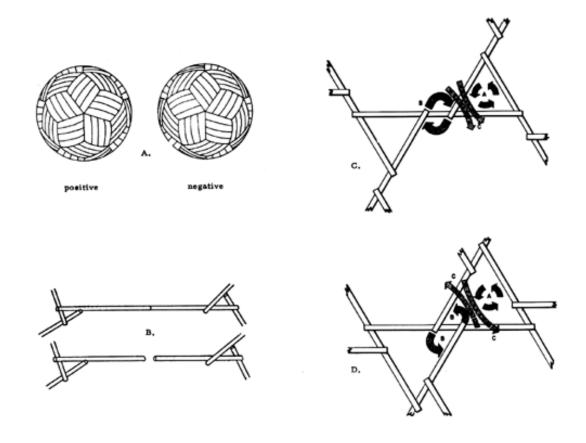
Fig. 770.11 System Turbining in Tensegrity Structures:
